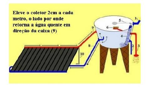
Support for fixing the solar collector
