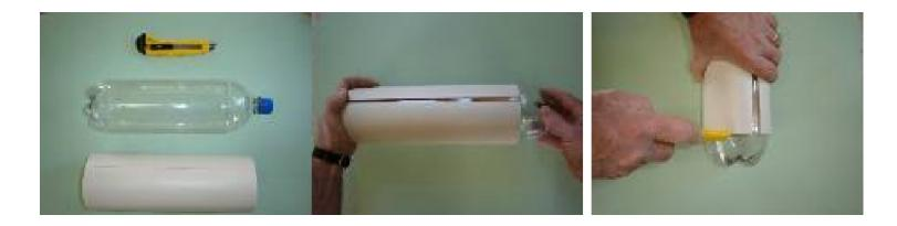
100 mm: 1 to 29 cm and the other with 31 cm and then make a cut lengthwise in 2 tubes, allowing the placing the bottle in it, defining the size of the cylinder to be cut. The pipe of 29 cm used for measuring the cutting of Lisas and bottles of Pepsi (new model) and the tube of 31 cm only for the cutting of bottles of Coke.
