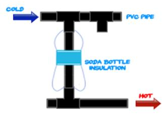
The standard solar water heaters cost a couple of 1000\$ and have copper as a main element. The Plastic Bottle solar water heater cost almost 50 \$ and is based on the thermosyphon technology which is used in many solar water heaters. It makes use of the circulation of water based on density; hot water which is less dense moves upwards while the cold water which is denser moves down. As long as the possibility of installation of the collector
